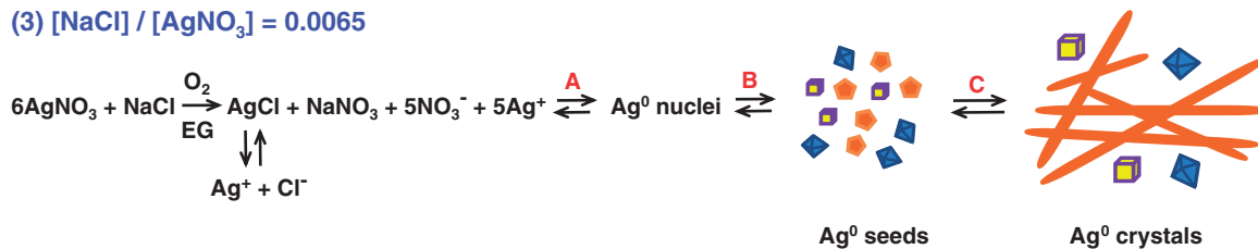
Scheme 1. Possible nucleation and growth mechanisms of Ag nanostructures at different molar ratios of [\text{NaCl}]/[\text{AgNO}_3] .
